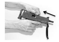
2 While holding cocking knob, pull trigger and ease bolt forward into closed position.
