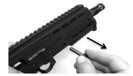
3 Remove upper receiver from lower receiver.
