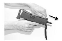
③ Remove front retaining pin and detach upper receiver from lower receiver.
