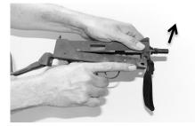
(4) Install Cocking Knob. Retract bolt until slot in bolt aligns with the rear of the slot in the upper receiver. Slide in cocking knob until it seats. Slide bolt and cocking knob forward.
